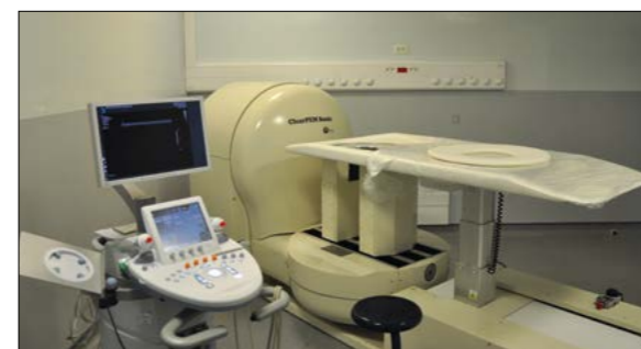
ClearPEM-Sonic installed at Hôpital Nord in Marseille, showing the ultrasound system (left) and ClearPEM system (right).
