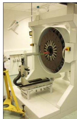
(Below left) ClearPET cassettes used in the PLANTIS project at Jülich. (Right) View inside ClearPET Neuro in Jülich, which was based on technology from CC and uses 20 cassettes containing crystal modules to image small animals.
