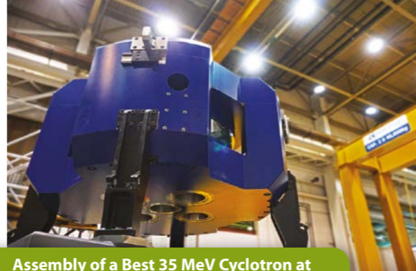
Assembly of a Best 35 MeV Cyclotron at Best Theratronics facility, Ottawa, Ontario, CA
