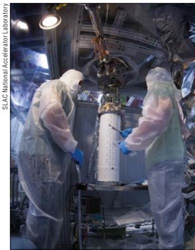
A mini version of the future LZ dark-matter detector at a test stand at the SLAC National Accelerator Laboratory, showing the detector TPC core (white container).
