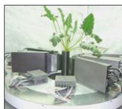
(Below left) ClearPET cassettes used in the PLANTIS project at Jülich. (Right) View inside ClearPET Neuro in Jülich, which was based on technology from CC and uses 20 cassettes containing crystal modules to image small animals.
