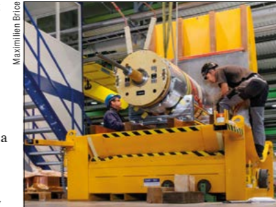
A model quadrupole magnet for the HL-LHC being prepared for cryogenic tests at CERN's SM18 facility in late September.
